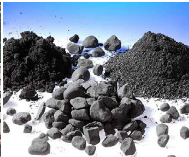
Vital ingredients: MaganDense magnetite aggregates
